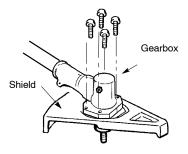
Insert and thread the 4 mounting screws through the holes of the gearbox and the metal shield. Tighten evenly and securely with the hex wrench provided.
